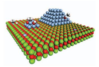
Figure 7.1: Schematic representation of supported catalytic particles. Image: Henrik Grönbeck.
