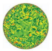
Figure 9.1: TCross-stream cut of turbulent pipe flow at high Reynolds number, showing colours of axial vorticity. The data was obtained from a high-resolution direct numerical simulation (DNS) using about 2.5 billion grid points. The fine scales close to the walls and the sharp gradients in the pipe centre are clearly visible which highlights the importance of adequate numerical methods and efficient codes. Image: Philipp Schlatter and George El Khoury.
